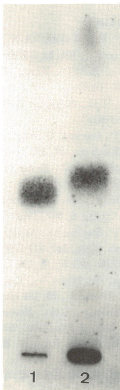
Fig.-5 Thin layer chromatogram of the ceramide produced from P. l. armigera sphingoethanolamine after hydrolysis by Cl. perfringens phospholipase C. Lane 1, authentic ceramide obtained from sphingoethanolamine of the green bottle fly, L. caesar ; Lane 2, ceramide obtained from sphingoethanolamine of the millipede, P. l. armigera . The plate was developed with chloroform-methanol (90:10, v/v). The spots were visualized with 50% H 2 SO 4 .
