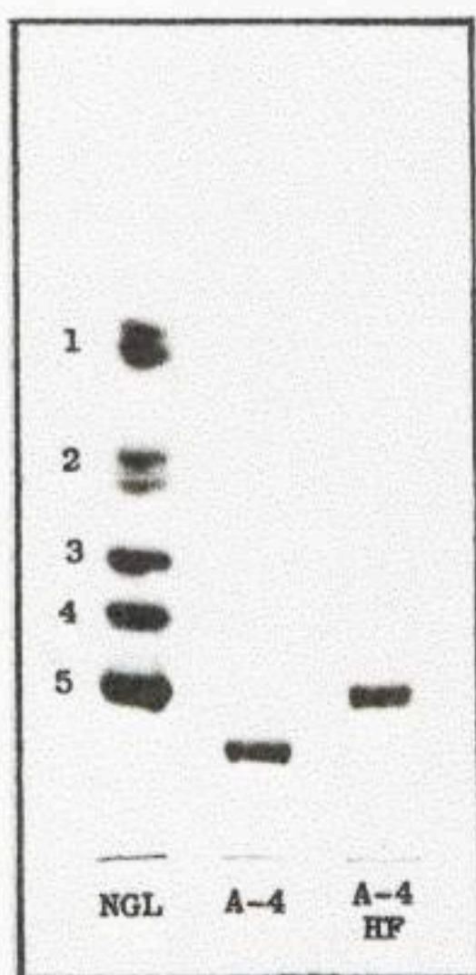
Fig. 5. Thin-layer chromatogram of the degradation product of A-4 with HF. Conditions used were the same as in Fig. 2.
