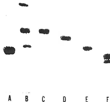
Fig. 11. Thin-layer chromatogram of several glycolipids. A, ganglioside from Tay-Sachs' brain; B, after hydrolysis of A with dilute HCl; C, guinea-pig erythrocyte mucolipid; D, human erythrocyte Globoside I; E, Globoside II; F, Globoside III. Solvent; chloroform: methanol: water, 60:35:8; Wako Gel B O, sprayed with anthrone-sulfuric acid
